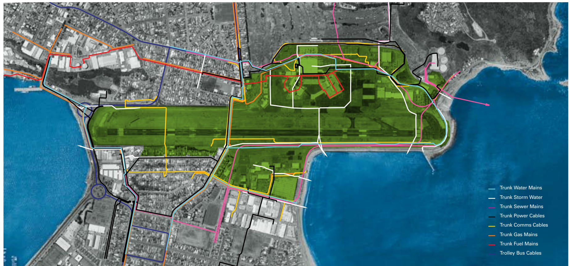
Figure 8-2 Alignment of Individual Trunk Reticulation Systems
