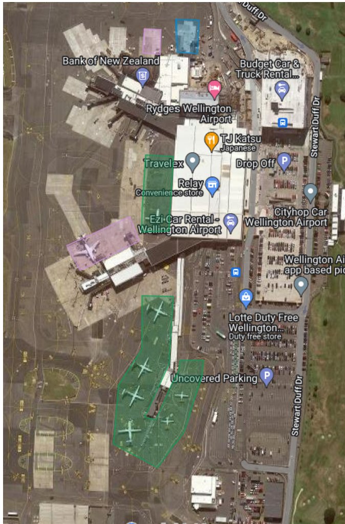
Figure 1: Electric GPU Stands at Wellington Airport. Green areas – Regional Gates where electric GPUs are available and consistently used, mauve area – Jet aircraft stands with electric GPUs available; and blue area – where the cabling and transformation equipment has been installed, however there is no electric GPU at this stage.
